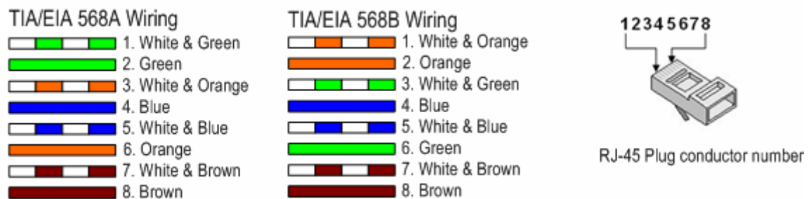
Picture 19 RJ45 Cable color code
